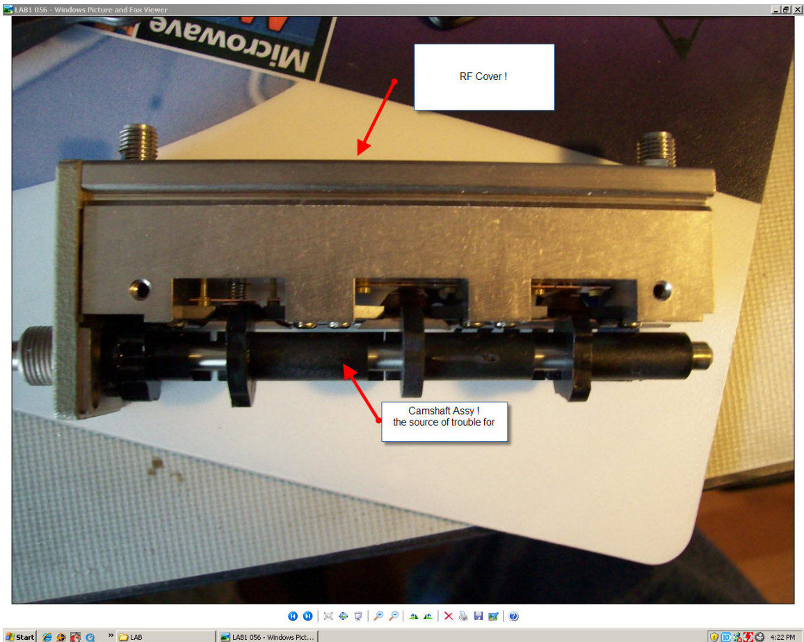
Side view showing the RF Cover and camshaft assembly, the camshaft wears out over time which causes failures, the RF cover holds the attenuators.
