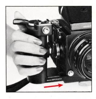
1) Pull out the film winding crank's attachment rod, while holding the film winding lever with the other hand. Then pull off the lever. Finally, slip the attachment rod back into position.
