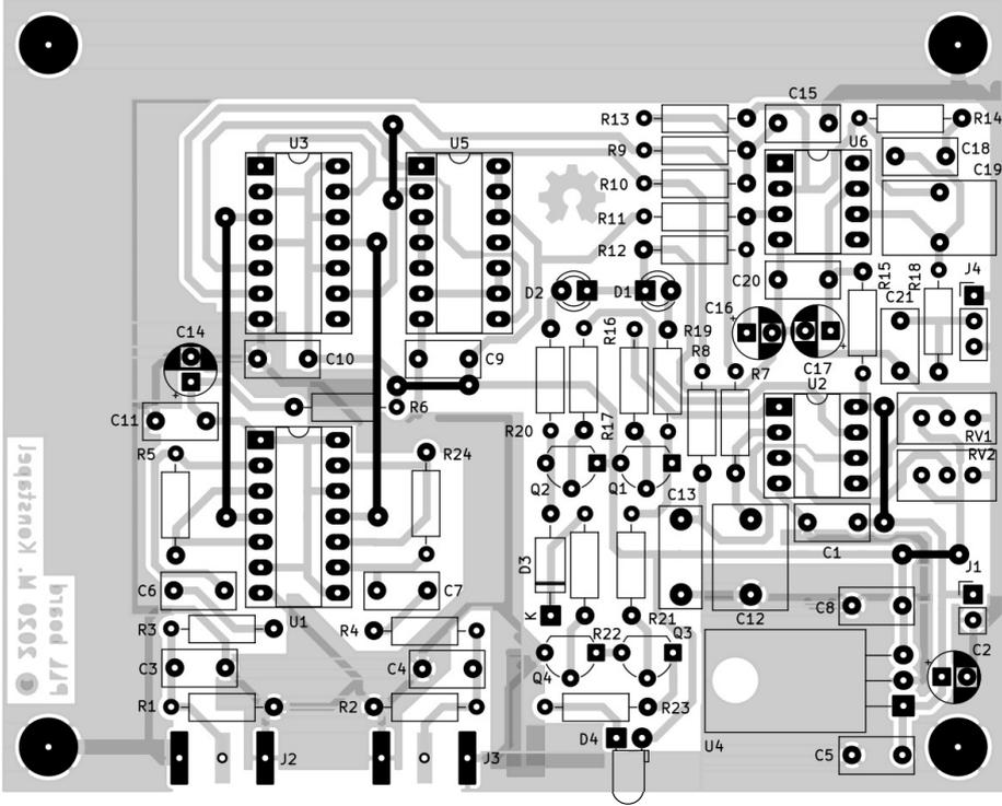
Figure 10: component placement
