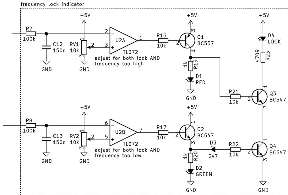
Figure 5: schematic of lock detector
