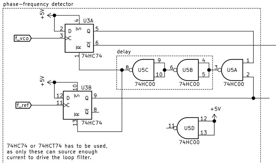
Figure 3: schematic of phase-frequency detector
