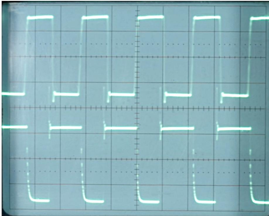
Figure 7: phase shift between reference oscillator and VCO
