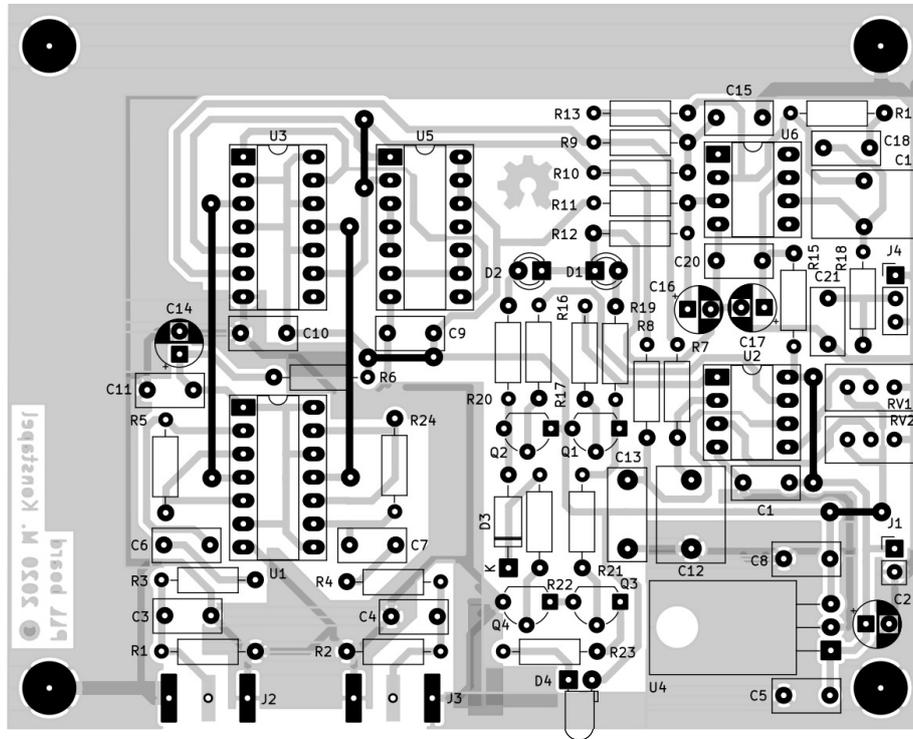
Figure 10: component placement
