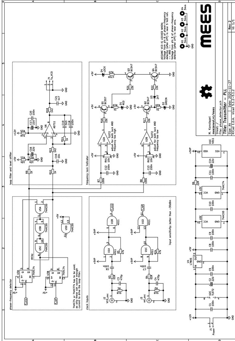
Figure 9: full schematic of PLL board
