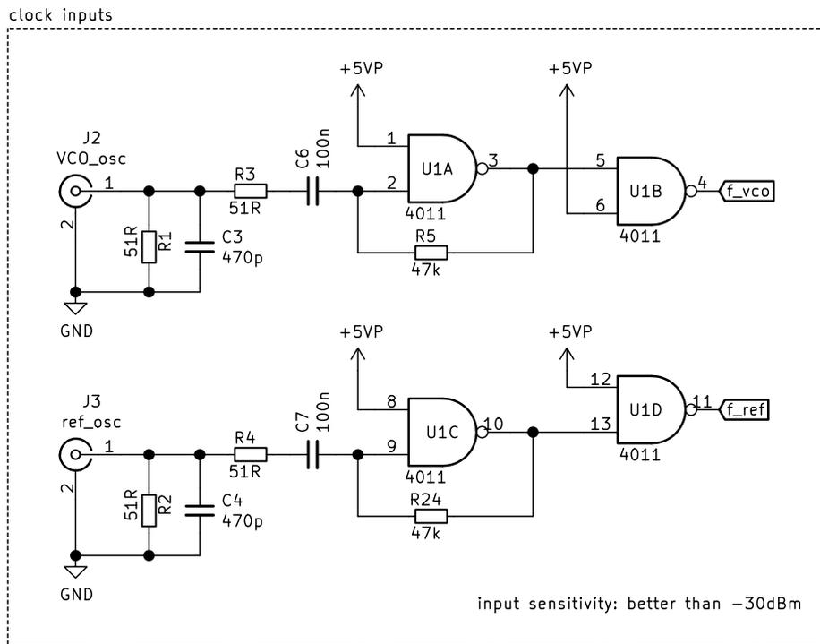
Figure 8: schematic of clock receivers
