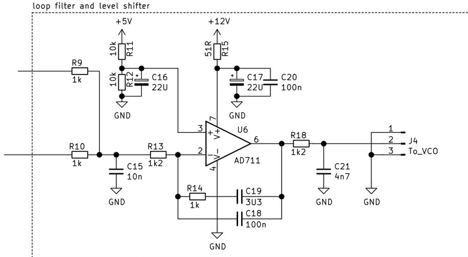
Figure 4: schematic of loop filter
