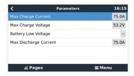
The 'charge current limit' (CCL) as shown in the parameters screen (and received from the BMS, by the GX device, via DVCC) will be the ceiling, and the system will try its best not to exceed that (as much as it can - it may spike under momentary peaking conditions).
