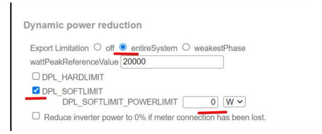
Then double check that all above criteria are met. It will show <u>Feed-in limiting active</u> **No** if the firmware requirement; the Data export; or the Sunspec Model type settings are incorrect, or the units are shut down (no available PV), or AC-input is disconnected / unavailable.
