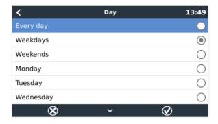
The Multi will start charging from the grid at the specified start time, and stop after the set duration or when the set SoC limit is reached. The period designated by the day, start time and duration will subsequently be referred to as a scheduled charge window
