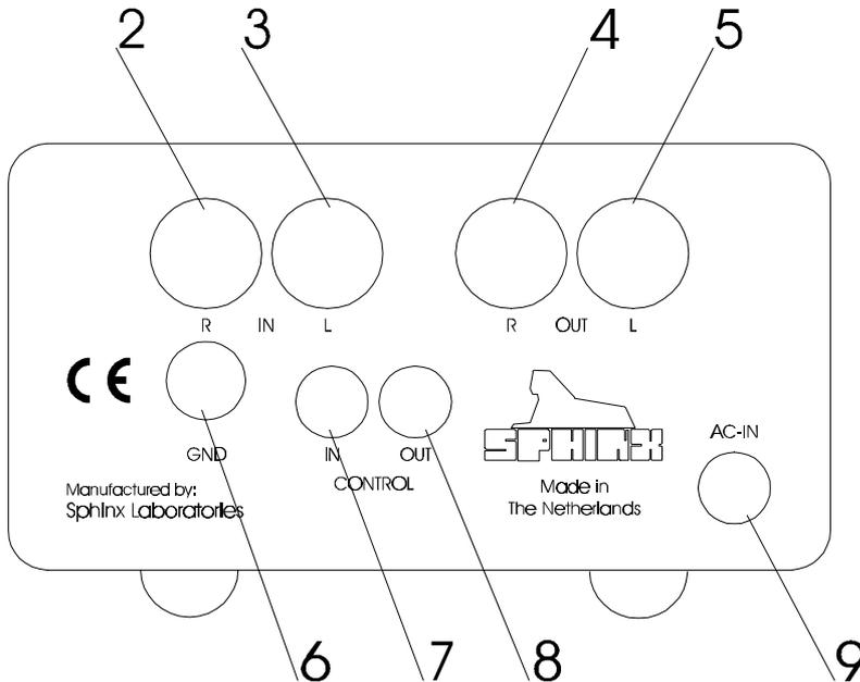
2. **R IN:** Connect to this input the *right* (red) output cable from the turntable.
