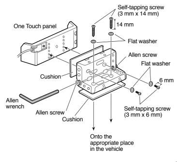
**Note:** Consider the safety of driver and passengers when deciding where to install the front panel. Tighten all screws firmly.
