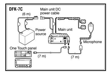
To install the microphone cable included with DFK-4C or DFK-7C, secure the microphone socket at the appropriate position in your vehicle using the long self-tapping screw (3 mm x 25 mm).
